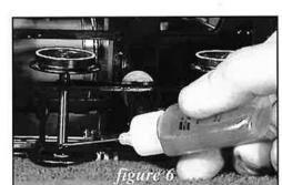
And be sure not to forget the lead truck bolster, where it interfaces with the screw attaching it to the cylinder saddle and locomotive frame.7
